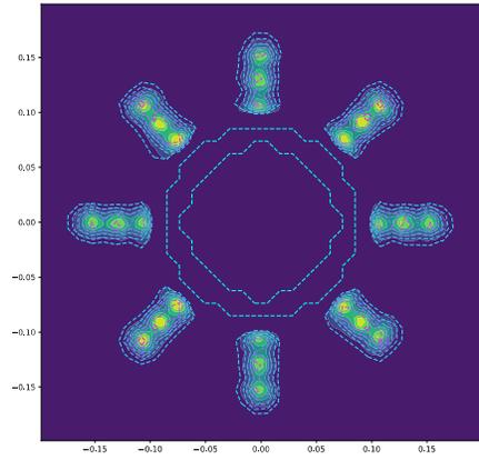
**Figure 16: Fine and coarse representations of the same total flux through a plane. The fine data were obtained from a simulation of the SKEC flare tip using 3mm resolution. It was coarsened to a 1cm resolution for the far field simulation.**
