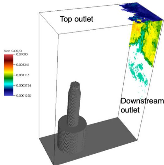
**Figure 4:  $\text{CO}_2$  distribution selected by 1 ppmv mixture fraction criteria at the outlet of simulation domain**
