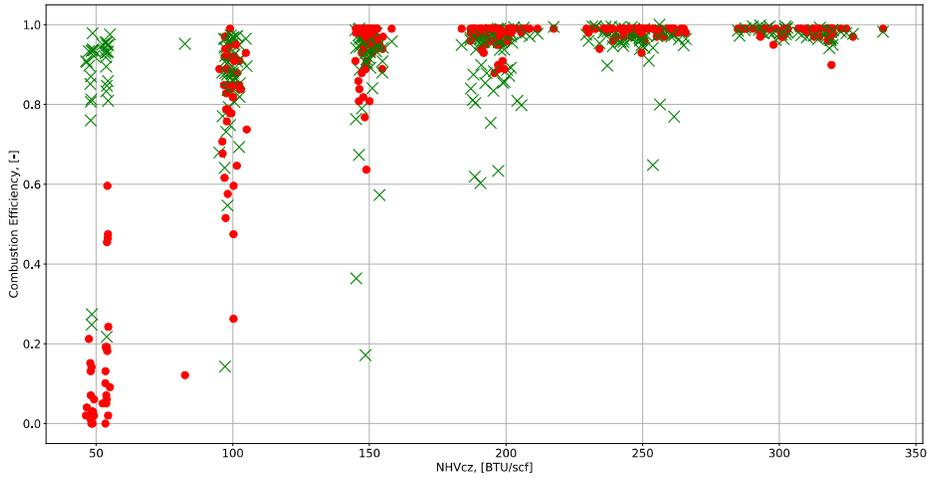
Figure 24: Means of the predictive posterior (red circles) compared against the measured data (green cross).
