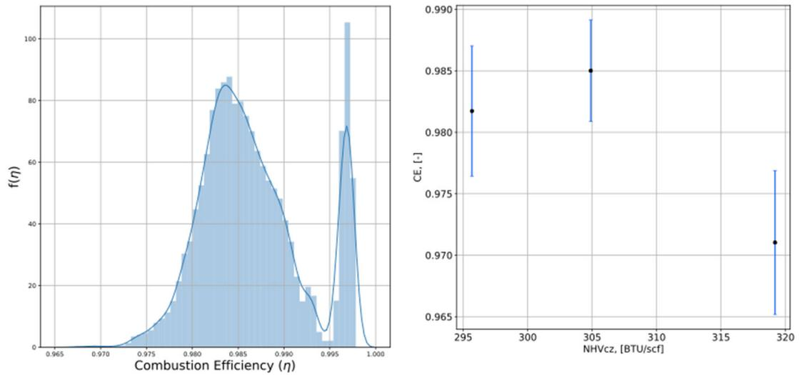
Figure 21: Predictive posterior for Case 1 (left) along with 95% confidence intervals (right) constructed from the measured data.
