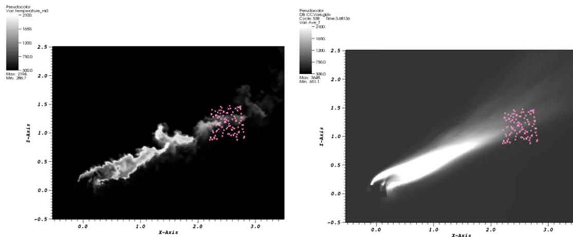
**Figure 7: Instantaneous (left) and time-averaged (right) LES temperature plots with the PFTIR instrument model target samples shown with pink markers.**
