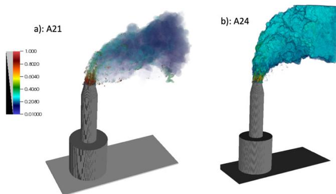
**Figure 12: Volume rendered image of stripping factor assessment for A2.1 and A2.4 simulation**
