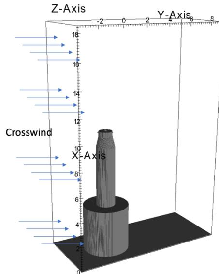
**Figure 2: Full-scale simulation domain for air-assisted flare**
