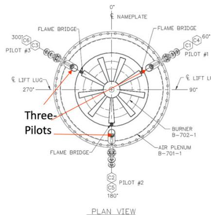
Figure 1: Three-pilot configuration for air-assisted flare
