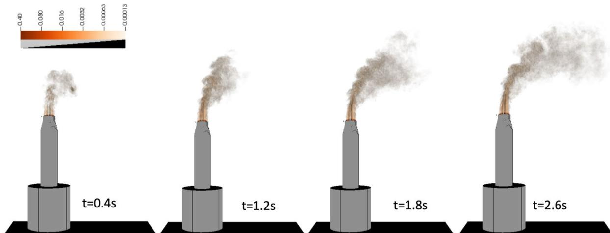
**Figure 11: Temporal evolution of unsteady CO<sub>2</sub> mass fraction field for full-scale simulation of A2.4**
