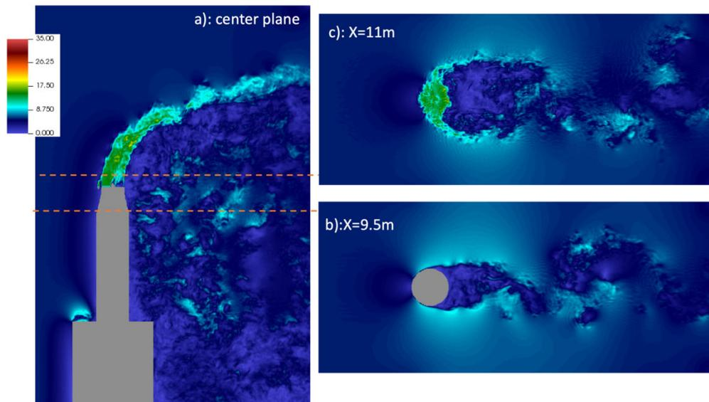
Figure 8: Velocity Magnitude distribution for A2.1 flare simulation: a) center plane, b)  $X=9.5$  m plane, c)  $X=11$  m plane
