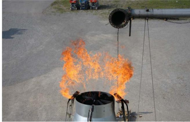
**Figure 3: Air-assisted flare tip with sampling collector in TCEQ 2010 test**
