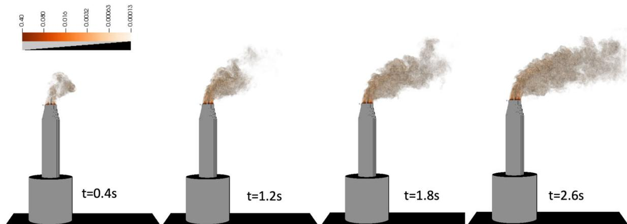
Figure 10: Temporal evolution of unburned fuel mass fraction field for full-scale simulation of A2.1
