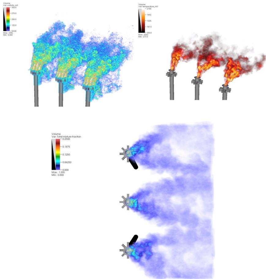
**Figure 17: Volume rendered images of the coarse level simulations using the fine level information. Here we show vorticity (top-left), temperature (top-right) and total mixture fraction (bottom).**
