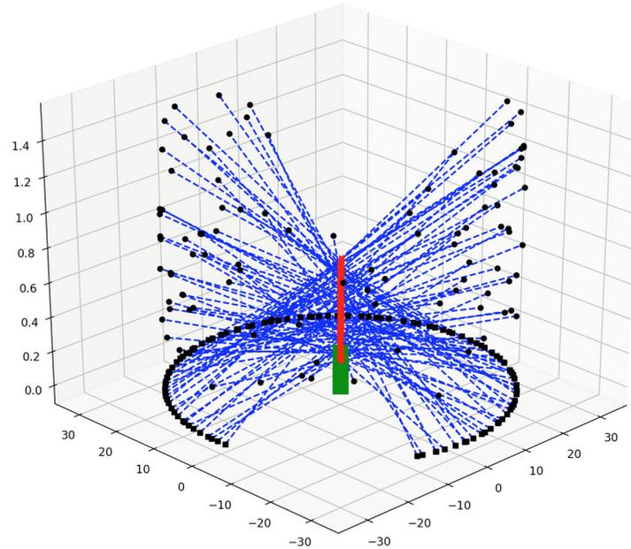
**Figure 6: Example of the PFTIR instrument model sampling showing the variation in the targeting position and the wind direction effect. The flare stack is indicated with the green bar. The intersecting targets are shown with red dots. The starting and stopping locations of the PFTIR ray are indicated with black dots while the ray path is shown with the dashed blue line.**
