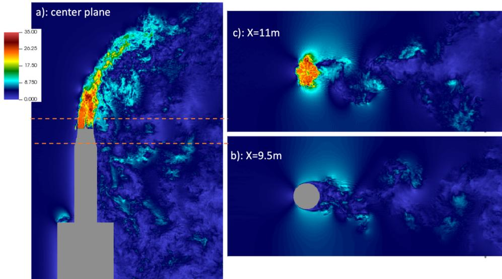
Figure 9: Velocity Magnitude distribution for A2.4 flare simulation: a) center plane, b) X=9.5m plane, c) X=11m plane
