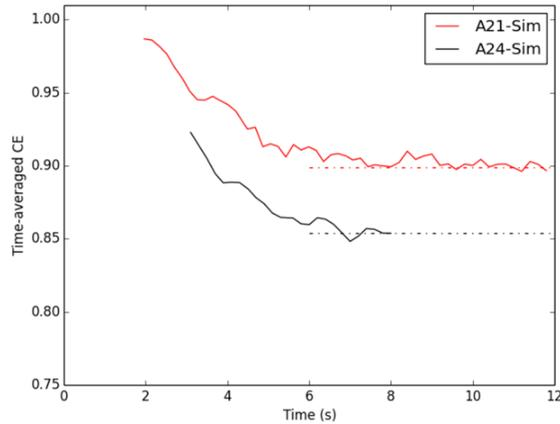
**Figure 14: Temporal evolution of time-averaged combustion efficiency at flare plume**
