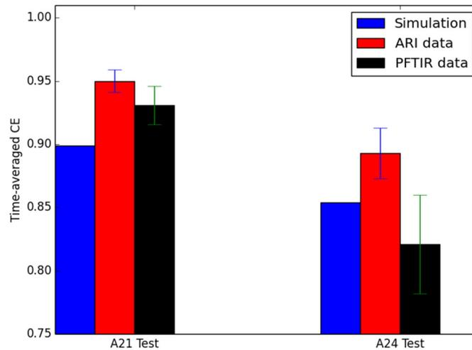
Figure 15: Comparison of measured and predicted combustion efficiency
